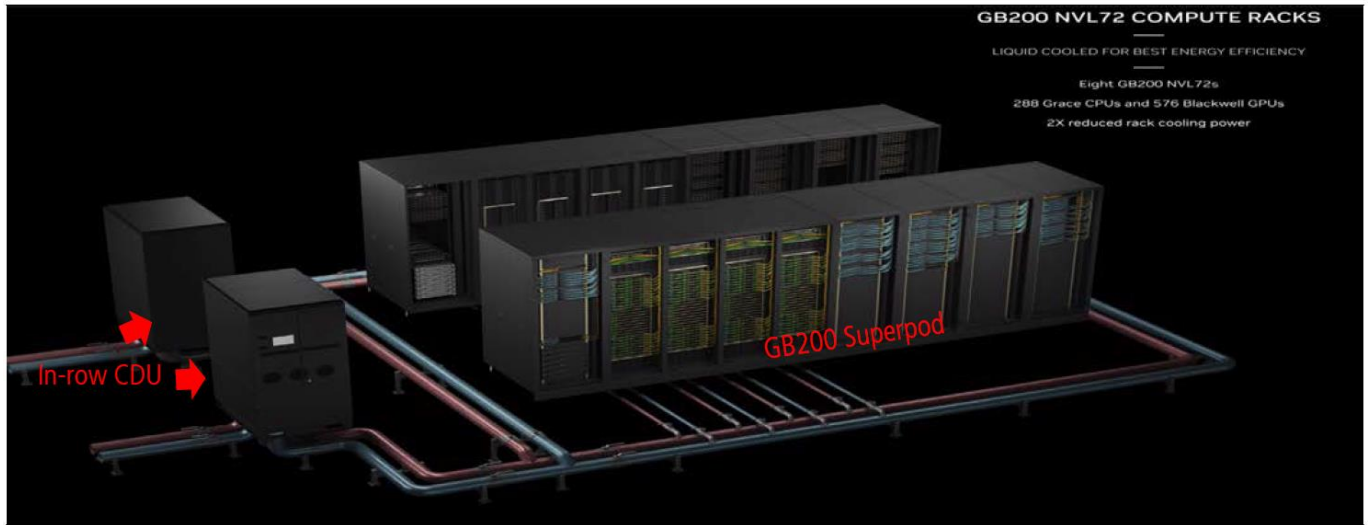
Figure 10: GB200 Superpod – Contains 8 NVL72 racks
