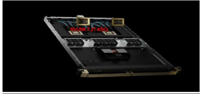
Figure 8: Each GB200 switch tray includes two Nvlink chips
