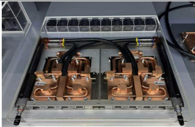
Figure 47: Delta offers cold plate and thermal fan solutions for GB200 servers
