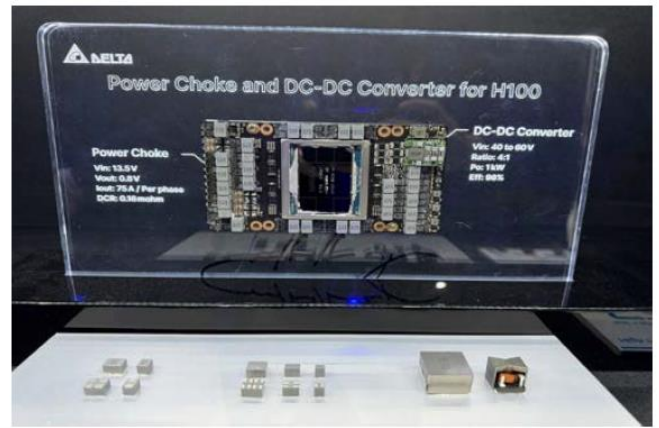
Figure 46: DC-DC power converters and chokes are upgraded on AI servers migrating from 12V to 48V
