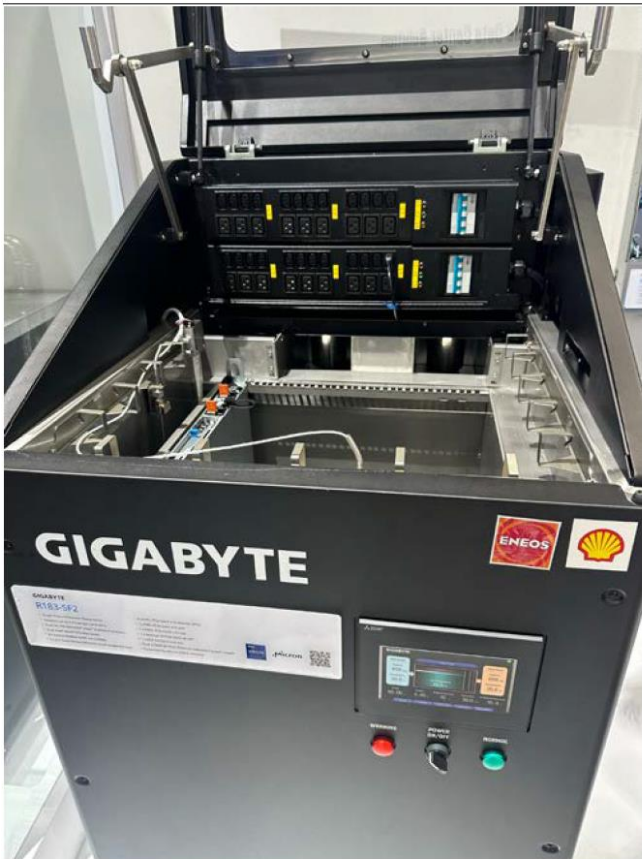
Figure 42: Gigabyte's immersion cooling tank
