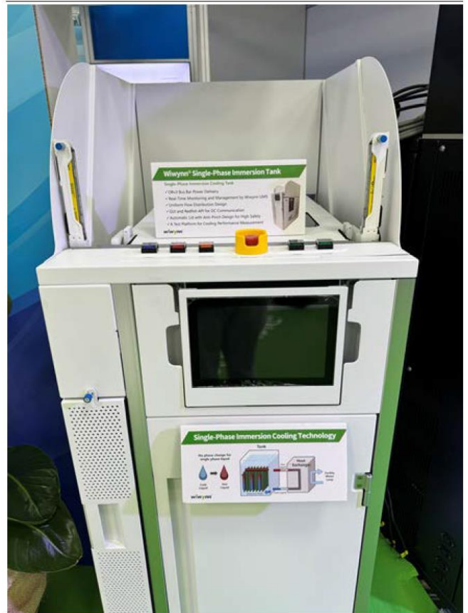
Figure 35: Wiwynn's single-phase immersion tank
