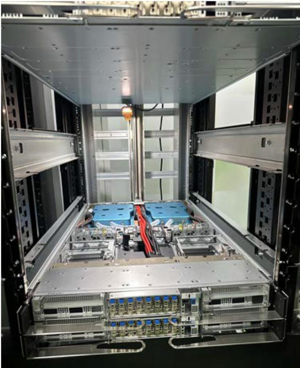
Figure 28: Wiyynn's 2-PDLC (two-phase liquid cooling) cold plate
