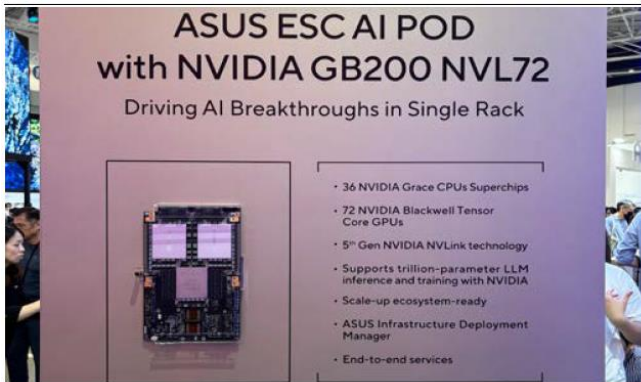
Figure 57: The compute tray of ASUS' ESC AI POD for the NVIDIA GB200 NVL72
