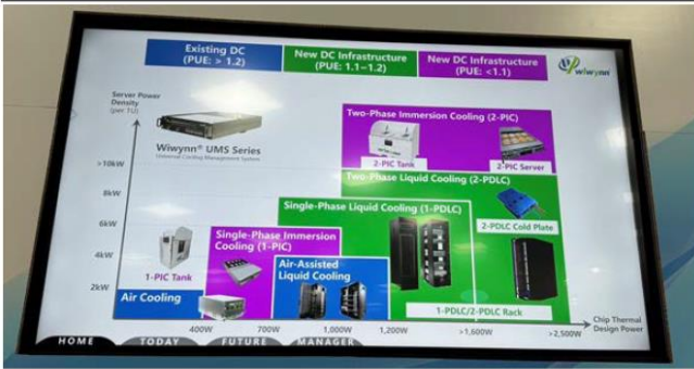
Figure 30: The server power density and chip thermal design power matrix of Wiyynn’s solutions
