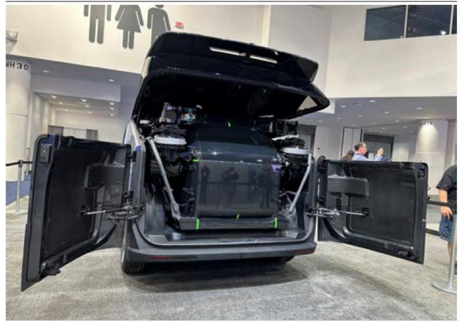
Figure 31: Air module of Xpeng Aeroht is stored in the rear cabin of a ground module
