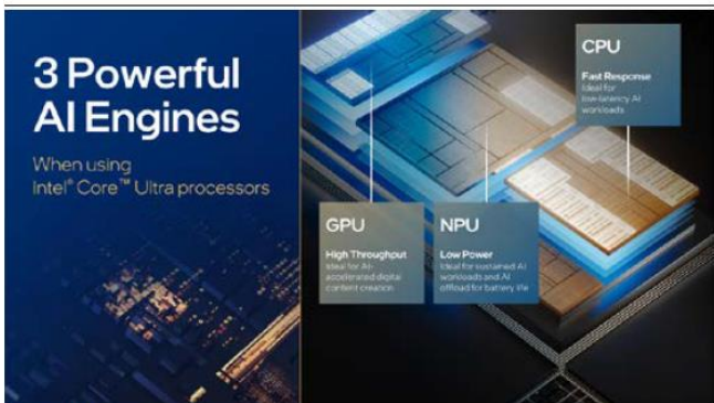
Figure 7: Intel Core Ultra CPU, Meteor Lake, integrates a CPU with an NPU & GPU
