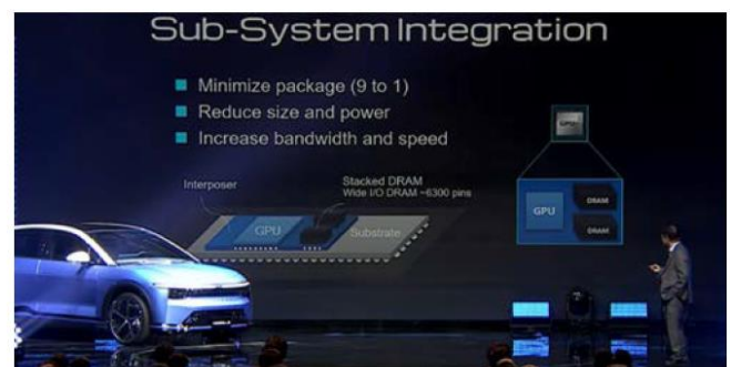
Figure 22: Subsystem integration can minimize packaging & reduce size and power under increased bandwidth and speed
