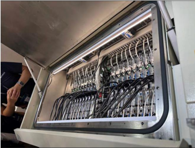
Figure 27: Single-phase immersion cooling technology
