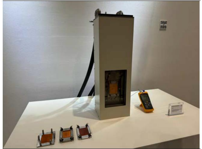
Figure 28: Two-phase immersion cooling technology
